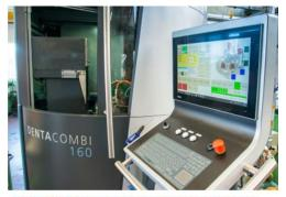
The DentaCombi 160 is a fully automated machine designed for multi-shift operation.
