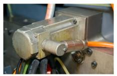
Motors from the AKM Washdown range position the grinding tool as robust units. Less space, less weight fewer installation masses need to be moved in the system thanks to the single-cable connection technology.
