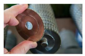
Alesa has developed its own machine to grind the teeth on the circular saw blade.
